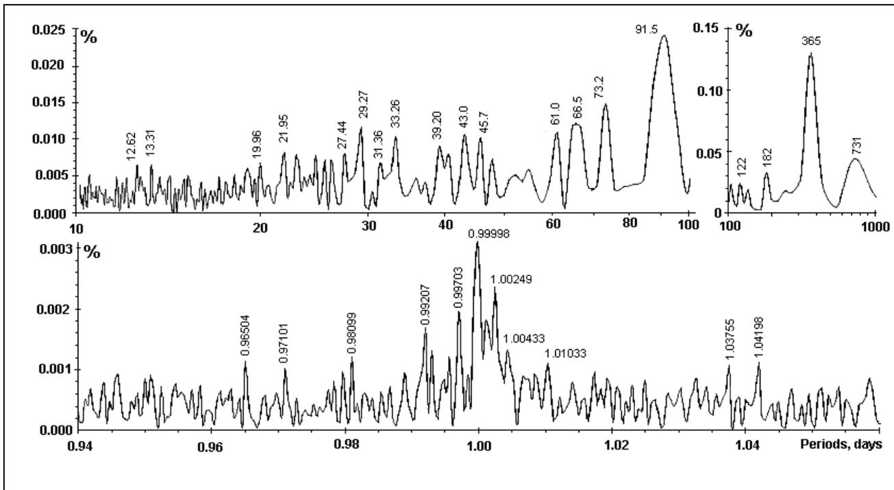
**Fig. 3.** Periodograms of count rate variations for the  $^{90}\text{Sr}$ - $^{90}\text{Y}$   $\beta$  source with the G-M counter CBM-12. The corresponding data were recorded between April 2000 and March 2007. Amplitude deviations are shown as percentage of the average count rate [3, 5]. The numbers near the peaks represent values of the corresponding periods in days.
