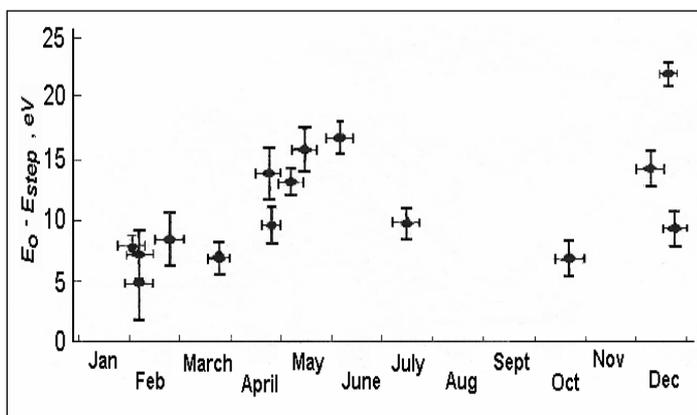
**Fig. 6.** Results of the Troitsk experiment [6]. Annual dynamics of the difference between theoretical and experimental segments of a spectrum of tritium  $\beta$  decay near the maximum electron energy (1994-2001).
