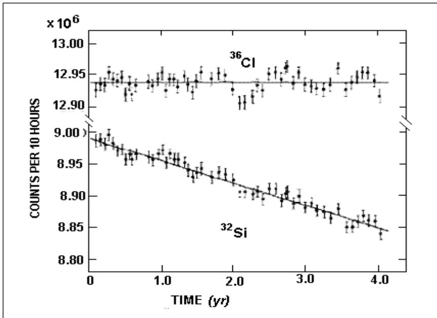
Fig. 7. Periodic changes in count rates for  $^{32}\text{Si}$  and  $^{36}\text{Cl}$  [1]
