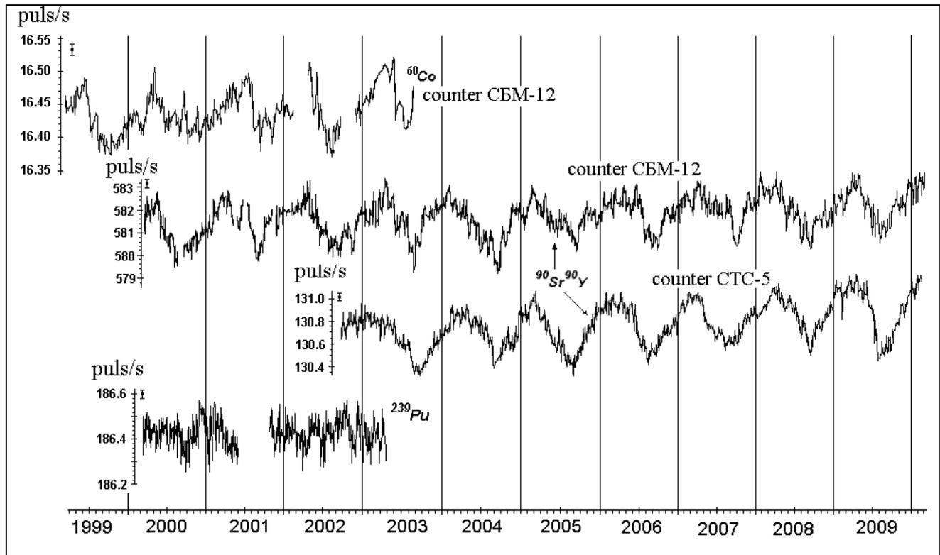
**Fig. 1.** Count rates for  $^{60}\text{Co}$  and  $^{90}\text{Sr}-^{90}\text{Y}$   $\beta$  sources measured by G-M counters, adjusted for a decrease in source activity with half-lives of 5,27 and 28,6 years, and count rate for  $^{239}\text{Pu}$   $\alpha$  source measured by the silicon detector [3, 5].
