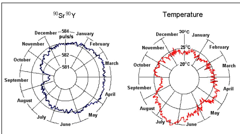
**Fig. 2.** Comparison of an average count rate for  $^{90}\text{Sr}-^{90}\text{Y}$   $\beta$  source with temperature variations near the installation. The results obtained since April 2000 till March 2007 are treated.
