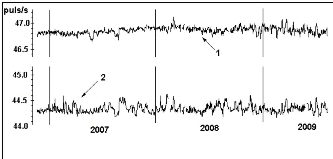
**Fig. 5.** Count rates for one  $^{239}\text{Pu}$   $\alpha$  source, registered by two silicon detectors.
