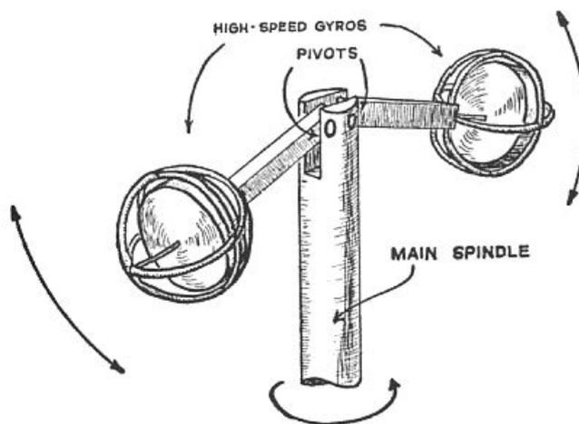
In the Laithwaite design, when the main axis rotates, the acceleration caused by the precession makes rise and fall the gyroscopes during each
