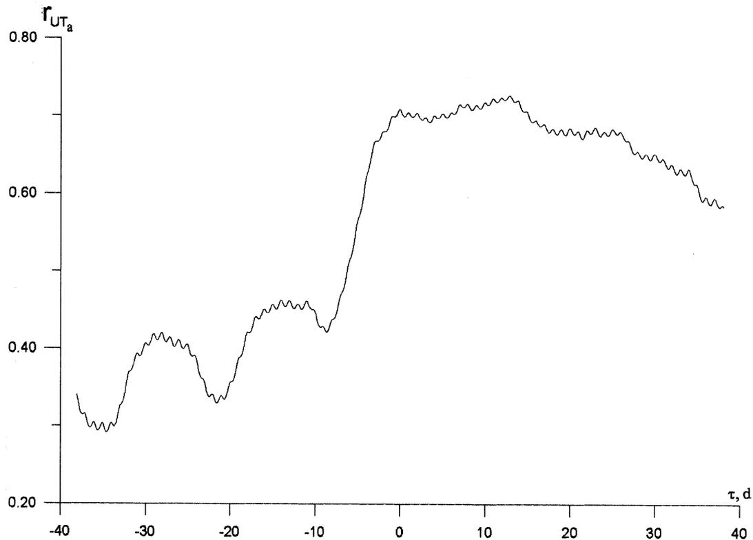
**Figure 1.** Correlation function of the detector signal  $U$  and atmospheric temperature  $T_a$   $r_{UT_a}$ . The  $t$  is time shift of  $T_a$  relative to  $U$  in days (negative  $t$  corresponds to retardation of  $U$  relative to  $T_a$ , positive  $t$  – to advancement).
