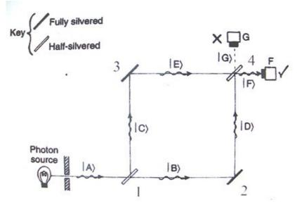
Figure 1. Quantum interferometer. Photon source - a source of photons; Fully silvered - completely reflecting mirror; Half-silvered - a translucent mirror («a divider of photons»); G and F - detectors of photons.
